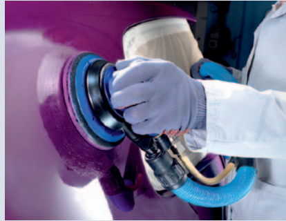
Producing a mat finish on painted surfaces
