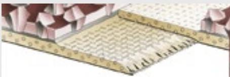
Overlapped joint with grit sanding
